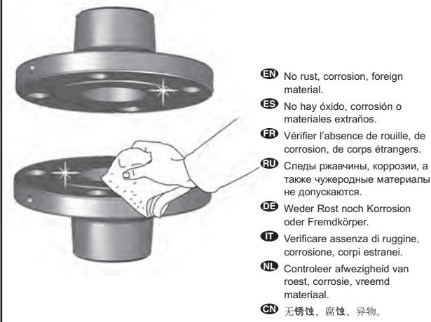
**EN** No rust, corrosion, foreign material.
