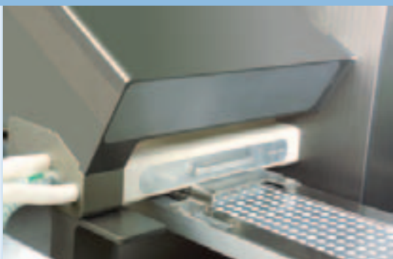
Precision filling: Drum filler for dosing powder quantities starting at 1 mg.
