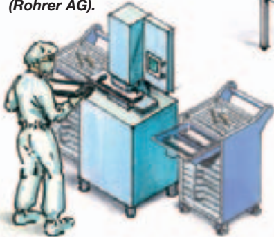
Machine for the forming, sealing and die-cutting of blister sheets (Rohrer AG).
